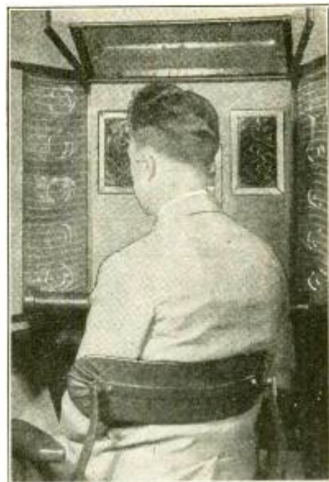
The two caesium-oxygen cells are mounted directly in front of the subject; note squares at either side of his head.
