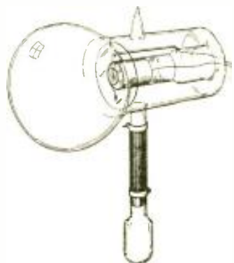
Above: The newest Bell Telephone Lab's., neon tube, having a concentrated or "crater" target, which provides a better image than before.
