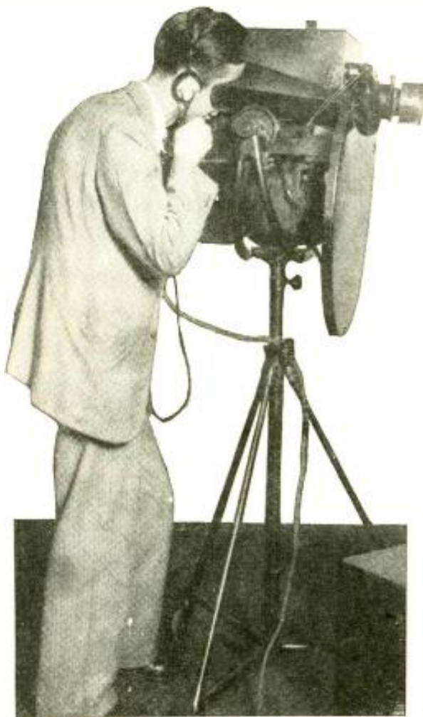
The television cameraman at work, focusing his picture by means of the "monitor" view-finder, while checking on his signals by means of head-phones.
